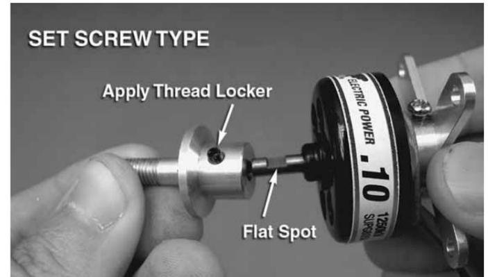
1. If you are installing the set-screw type of prop adapter, remove the set screw(s) from the base of the prop adapter and apply a drop of thread-locking compound to each set screw's threads. Fit the prop adapter to the motor shaft so that at least one set screw is aligned directly over the flat spot on the motor shaft. Slide the prop adapter all the way onto the motor shaft and tighten the set screw(s). The flat spot and set screw(s) will keep the prop adapter keyed to the motor shaft.
