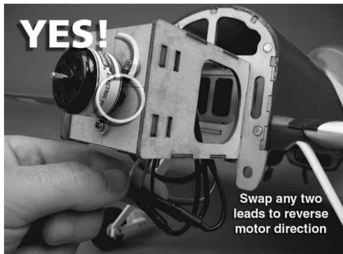
4. Mount your motor to the firewall using the screws, washers, and blind nuts supplied with your model kit. 4-40 sized hardware or 3mm hardware is adequate for these SuperTigre motors. If you are using the SuperTigre 370 or 400 motor, route the motor
