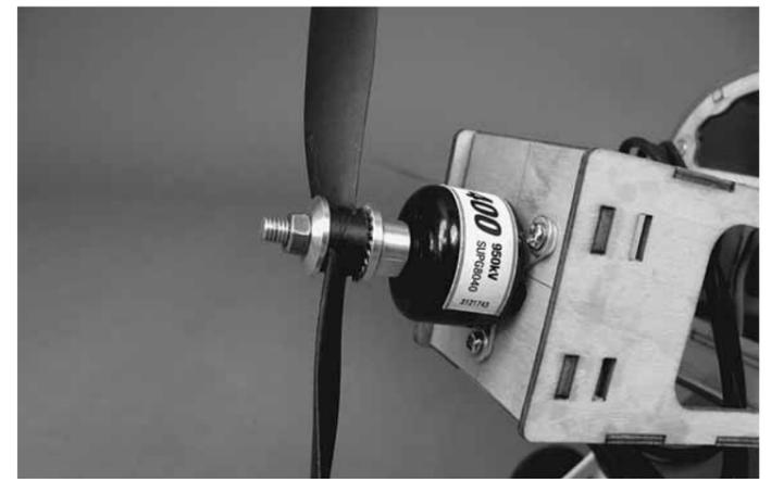
3. If your airplane has a cowl, install it now. Fit a balanced propeller to the prop shaft and install the prop washer and prop nut. Tighten the prop nut securely.
