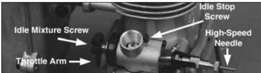
**High-Speed Needle:** The high-speed needle controls the amount of fuel entering the carburetor during medium and high speed operation.
