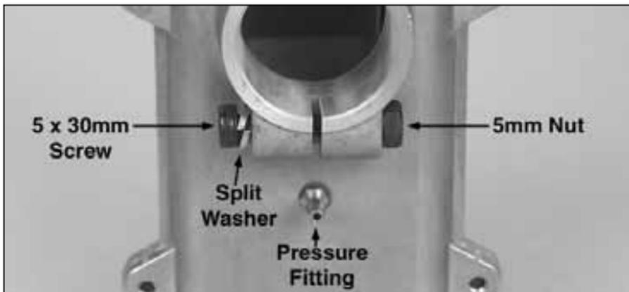
Install the 5mm x 30mm screw, split washer and 5mm nut in the muffler, but do not tighten. Slide the muffler over the
