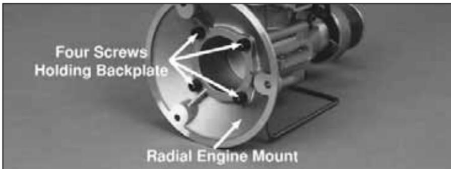
If the G3250 engine is to be mounted on the radial mount provided with the engine, remove the four screws holding the backplate. Remove the rubber O-ring on the backplate and install it on the radial mount. Attach the radial mount to the engine using the four longer screws and split washers provided. Install the radial mount to the firewall of the airplane with three 8-32 screws, three split washers and three blind nuts. (Not Included.)
