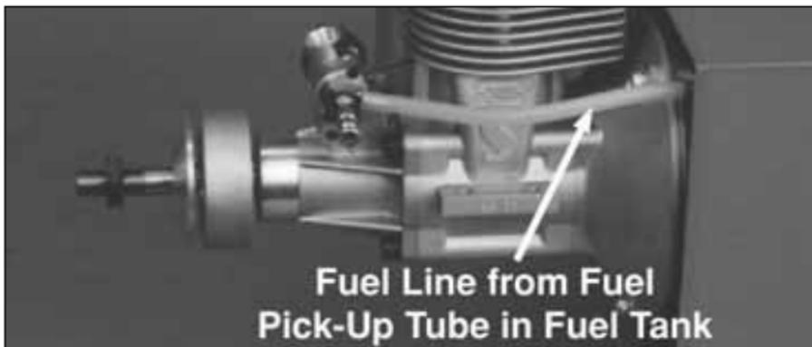
Connect a medium or large size silicone fuel line from the fuel inlet on the carburetor to the fuel pick-up tube that is connected to the clunk in the fuel tank. We suggest that a fuel filter be installed in the fuel line between the carburetor and the fuel tank. The filter will prevent any contaminants in the fuel from clogging the carburetor.
