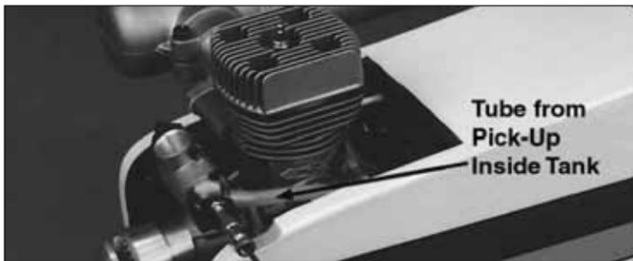
Connect a medium size (3/32") silicone fuel line from the fuel inlet on the carburetor to the fuel pick-up tube that is connected to the clunk in the fuel tank. We suggest that a fuel filter be installed in the fuel line between the carburetor and the fuel tank. The filter will prevent any contaminants in the fuel from clogging the carburetor, or damaging the engine parts.
